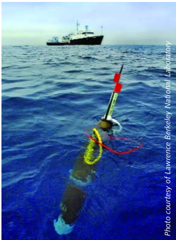
Carbon Explorers are ocean floats with carbon sensors, enhanced communications, and remote programming capacity. They are enabling scientists to track variations in the ocean's carbon cycle year-round with unprecedented accuracy.
